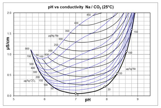
Figure 2. Conductivity and pH of mixtures of NaOH with  $CO_2$  solutions in high purity water, at 25 °C. Pure  $CO_2$  is represented by the left-side border curve, pure NaOH by the right one. Values in between are for mixtures.
