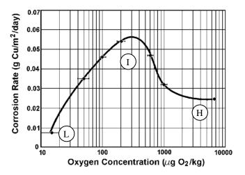
Figure 1. Copper release rate as a function of oxygen concentration [8]. L and H indicate the regions for low- and high-oxygen chemistry, respectively, and I the intermediate region.
