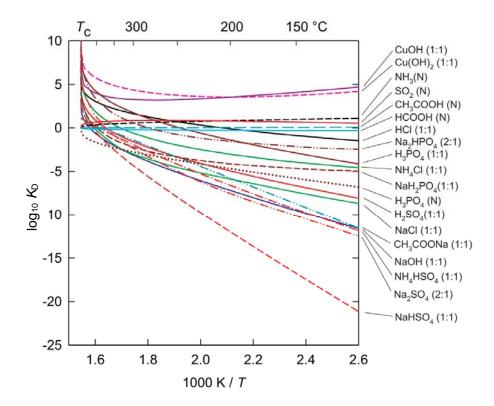
Figure 2. Partitioning constants (*K*<sub>D</sub>) for some species plotted against reciprocal temperature (kelvin). It should be noted that the volatility of neutral (N) compounds can be compared directly with other neutral compounds on this figure, 1:1 compounds with other 1:1 compounds, and 2:1 compounds with other 2:1 compounds. But neutral compounds cannot be compared directly with 1:1 or 2:1 compounds [1,2]. Other examples of distribution coefficients can be seen in references [1] and [2].
